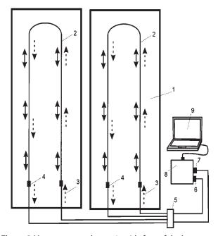
Figure 3 Measurement scheme: 1 – side face of the beam, 2 – optical fiber, 3 –direction of movement of the light wave through the sensors, 4 – connector, 5 – optical distribution frame for connecting patch cords, 6 – output adapter, 7 – input adapter, 8 – data processing unit, 9 – laptop with software
